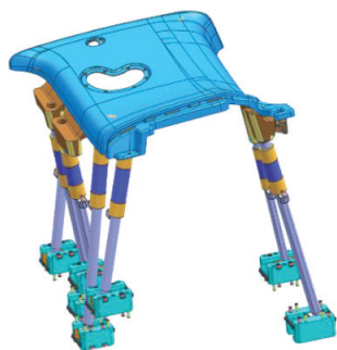
(b) Angle ejection pin and angle ejection block
